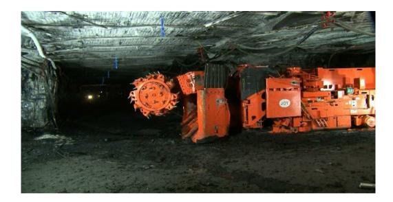
14ED25 Entry Driver Mid-seam, simultaneous mining and roof/rib bolting machine
