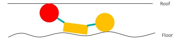
The absolute altitude of the shearer body is oscillating The shearer records the relative height of the lead drum to the lead shoe Shearer mode "extract to current" generates oscillations along the face
