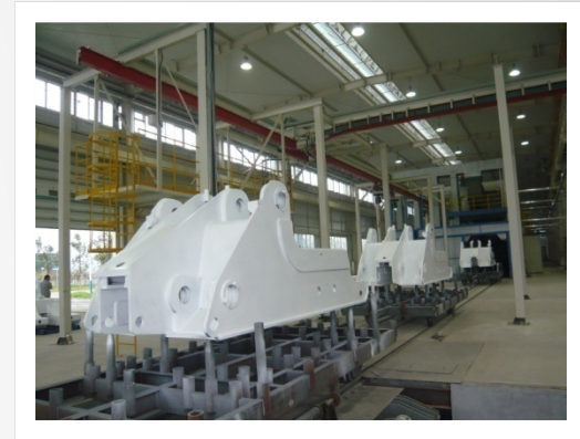
Spray painting of big structures
