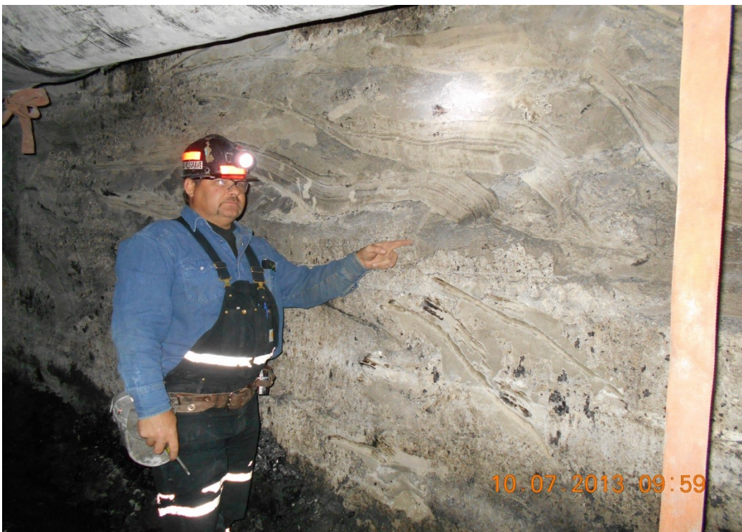
Looking at Phase 1 backfill from Phase 2 development
