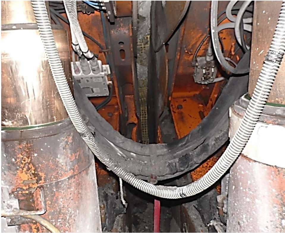
Huesker mesh (yellow) laid down behind the shields.
