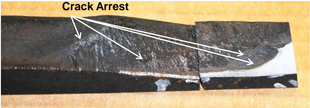
Crack tip of major crack in Head Gate end of Pan 71.
