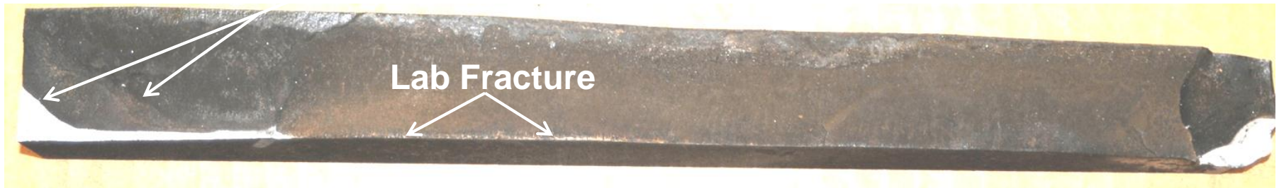
Pan 71 Tail Gate - Opened primary crack.
