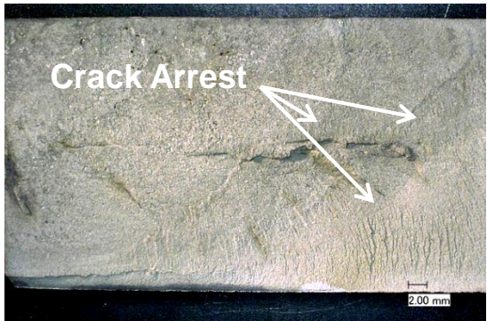
Crack tip of major crack in Head Gate end of Pan 71.
