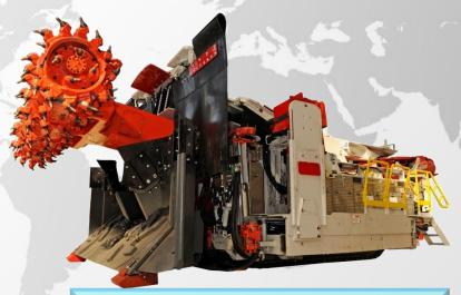
39 - 55 in (1 - 1.4 m) sump distance for increased bolt row distance
