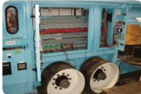
The ControlLogix® automation controller and PowerFlex® operator interface are mounted in the same control cabinet and communicate to the VFDs via Ethernet.
